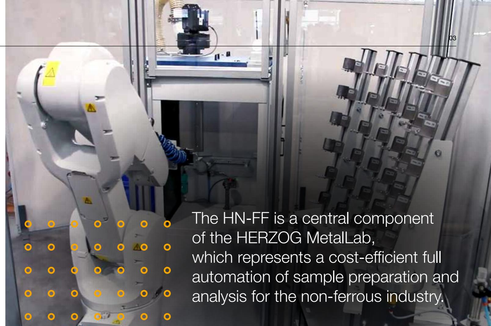
The HN-FF is a central component of the HERZOG MetalLab, which represents a cost-efficient full automation of sample preparation and analysis for the non-ferrous industry.
