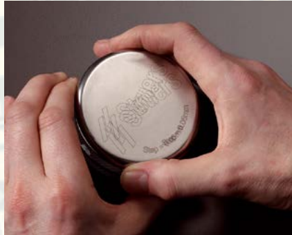
Controlled removal in steps of 50 µm
