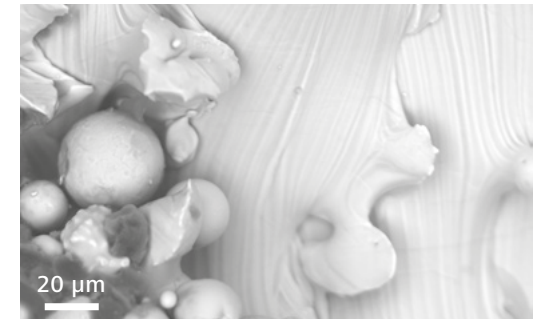
Surface of titanium alloy (Ti-6Al-4V) additively manufactured using selective laser melting, showing fully melted regions alongside unmelted Ti-6Al-4V particles and other material. Imaged with BSE detector on ZEISS EVO 15. Sample provided by TWI Ltd.
