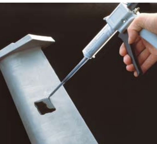
An operator dispenses RepliSet onto a sample
