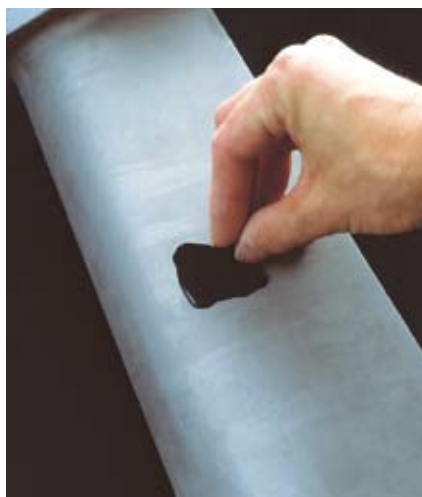
An operator peels off the cured replica
