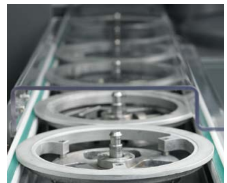
7. The finished specimen holder is moved to the conveyor, where it can be collected by the metallographer for microscopic examination
