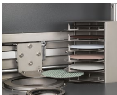
Step 3: ...and moves the MD-Consumable to the elevator.
