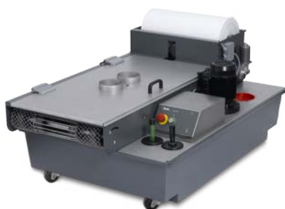
Coolimat-200 for Exotom-150, equipped with 200 l tank, band filter and Cooli-2 control unit.
