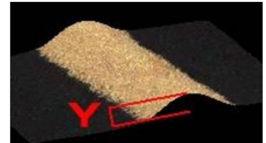
Silver finger: 3-D reconstruction on monocrystalline silicon solar cell;
