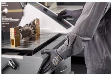
Two-hand safety operation with open hood
