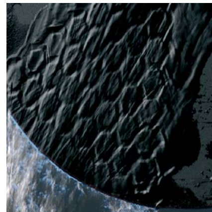
With the 3D surface all the water sprayed into the channels between the hexagons is transported into the cut, thus cooling the workpiece much more efficiently.
