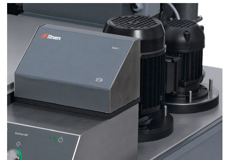
Coolimat-200 with two pumps and Cooli-1 control unit
