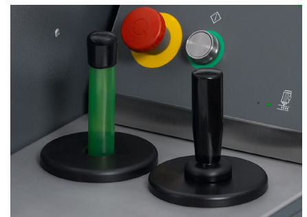
Coolant level indicator and optional magnetic filter (right).
