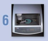
Mount TargetGrip in TargetMaster Lock TargetGrip into specimen mover of TargetMaster
