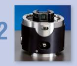
Lock into holder The specimen chair is locked into TargetGrip, a precision specimen holder
