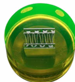
EpoDye, fluorescent dye to be mixed with the resin to allow for easy identification of pores and cracks when examining the specimen in fluorescent light.
