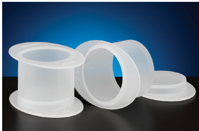
FixiForm is a two part mounting cup designed with practical handles to be as user-friendly as possible.
