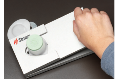
The mount is pressed carefully out of FixiForm
