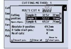
In MultiCut-4 both X- and Z-values for all cutting positions are recorded.
