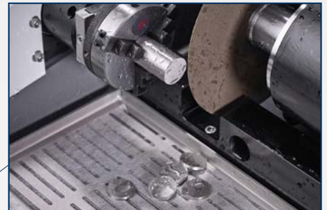
MultiCut function* provides extra productivity of up to 10 slices in a single workflow
