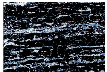
Structure of steel imaged in darkfield EC Epiplan 20x/0.4
